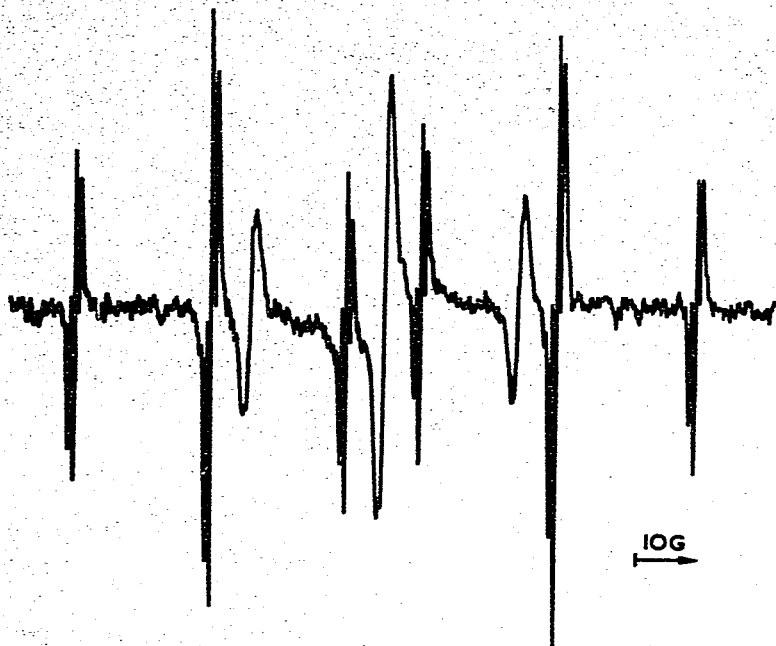
Fig. 1. ESR spectrum of the radical t\text{-BuOSnBu}_2\text{CH}_2\text{CH}_2\text{CH}_2\text{CH}_2 in cyclopropane at 153 K; a(\alpha\text{CH}_2) 21.9 G (2H), a(\beta\text{CH}_2) 28.0 G (2H), a(\gamma\text{CH}_2) 0.9 G (2H). For the corresponding diethyl compound the values are a(\alpha\text{CH}_2) 21.9 G (2H), a(\beta\text{CH}_2) 27.6 G (2H), a(\gamma\text{CH}_2) 0.9 G (2H) at 205 K.
